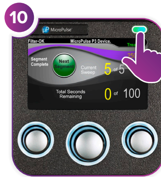
At completion of treatment, press this button to enter Standby Mode (disable laser).
