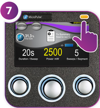
Press this button to enter Treat Mode (enable laser).
